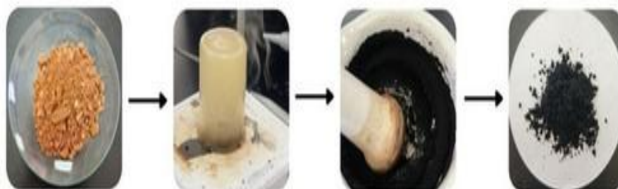
Fig 13: Eye liner (Kohl) manufacturing:
