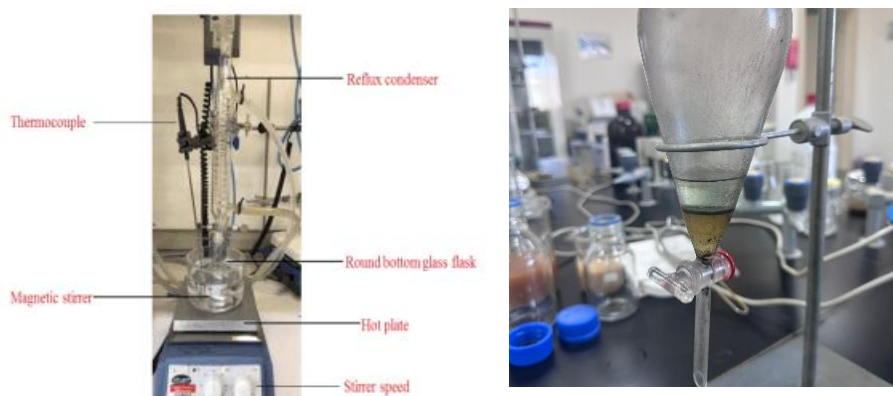
Figure 1: (a) Glass reactor for synthesis of biodiesel (b) Biodiesel separation After one-night stand biodiesel (the top layer) and glycerol.
